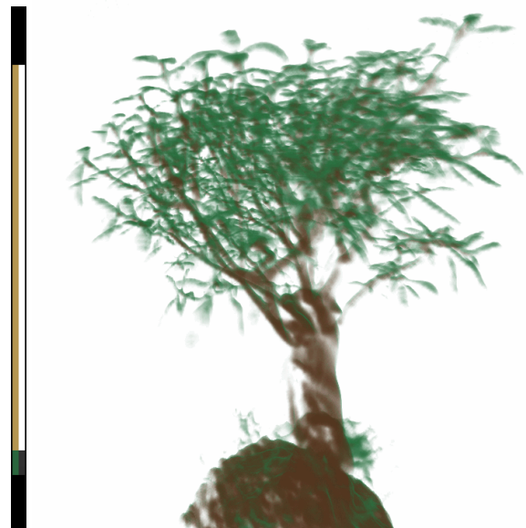
Figure 12: Hierarchical unstructured bonsai data set with approximately 1,200,000 tetrahedra rendered on an Apple iBook with our proposed multi-texturing technique. The transfer functions are depicted besides.
